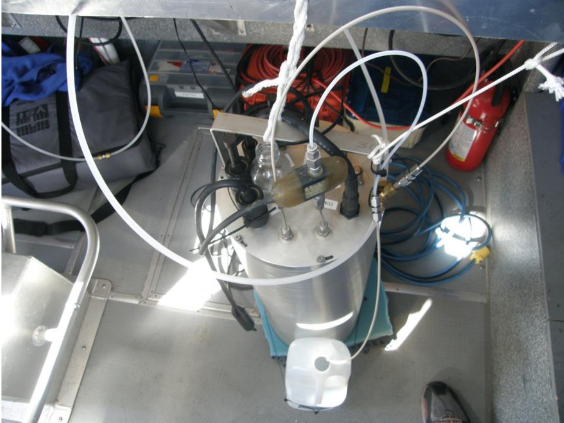
Fig. 18. The SRI Underwater Mass Spectrometer inside the cabin of the R/V CHINOOK.
