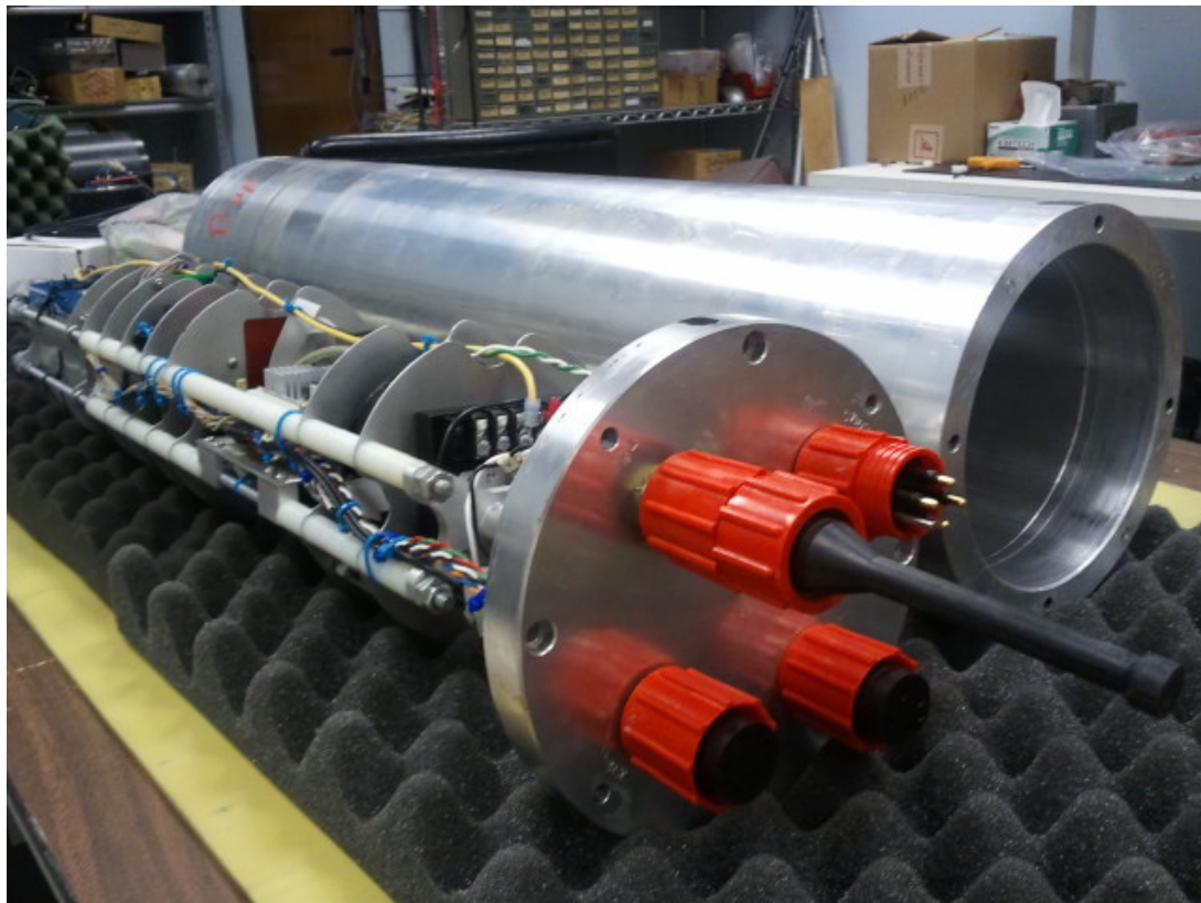
Electronics and housing for the Shallow Sediment Velocity Probe, SSVP.
