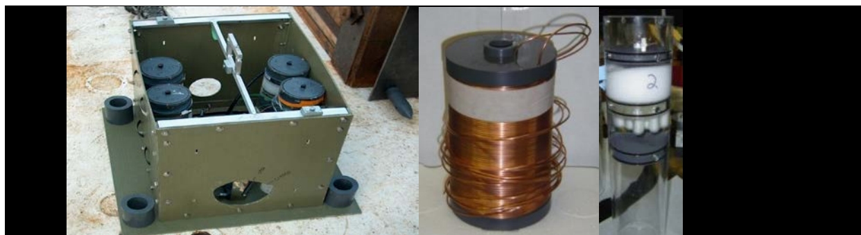
Figure 1. A fully constructed OsmoSampler package. The copper coil stores sample until package retrieval. This size copper coil is sufficient to hold ~10 months of samples. Four coils and osmopumps per package allow up to four sediment depths to be monitored simultaneously.
