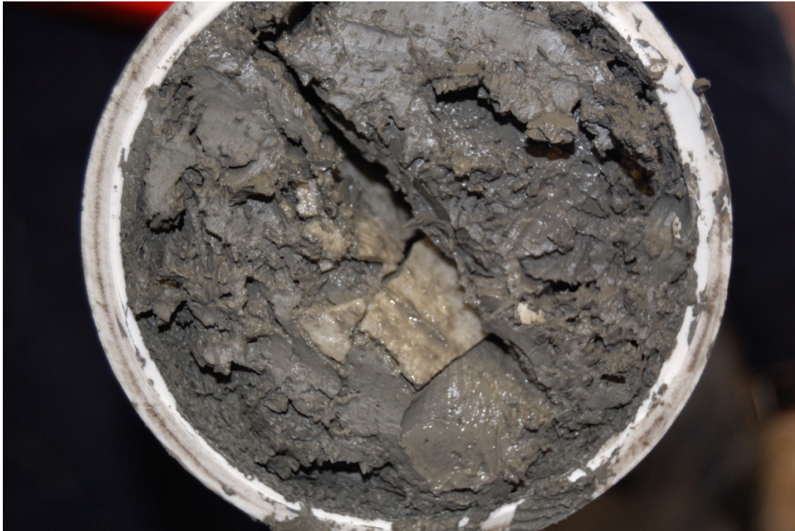
Chunks of hydrate 6 feet from the base of JPC-001.
