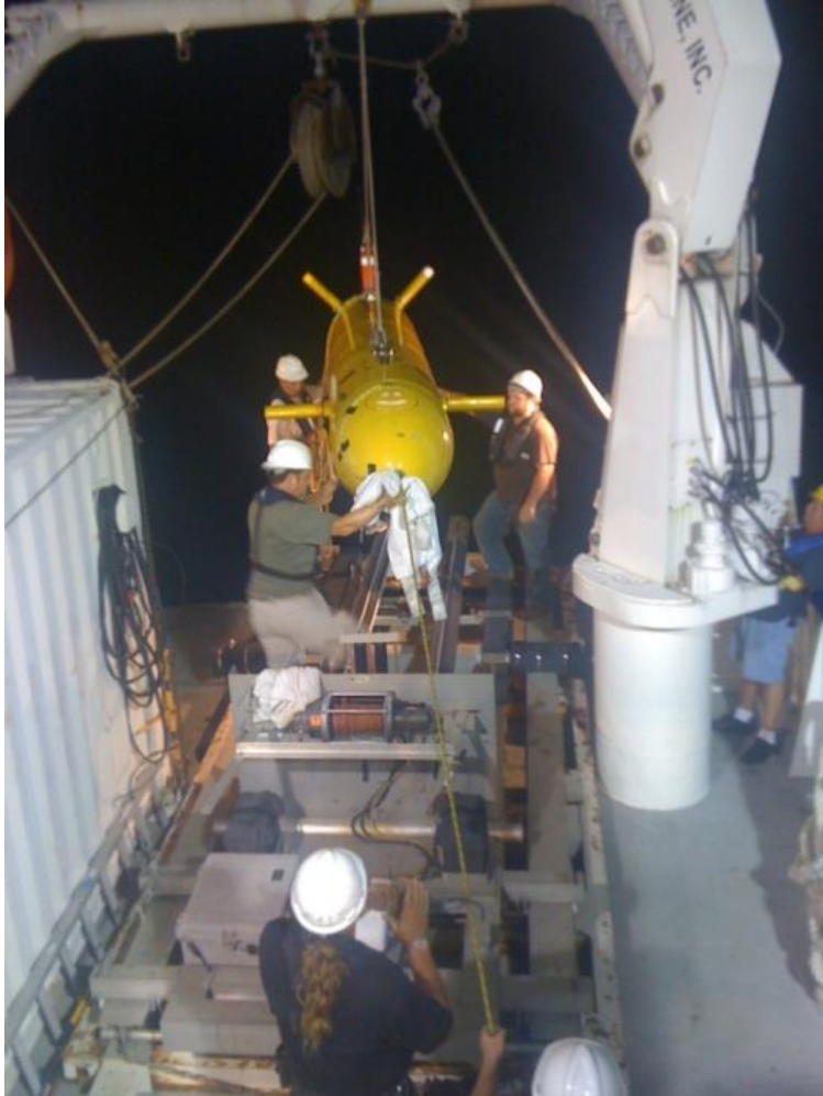
Figure 34. The AUV team prepares to launch the Mola Mola photo-AUV from the Pelican's upper deck.
