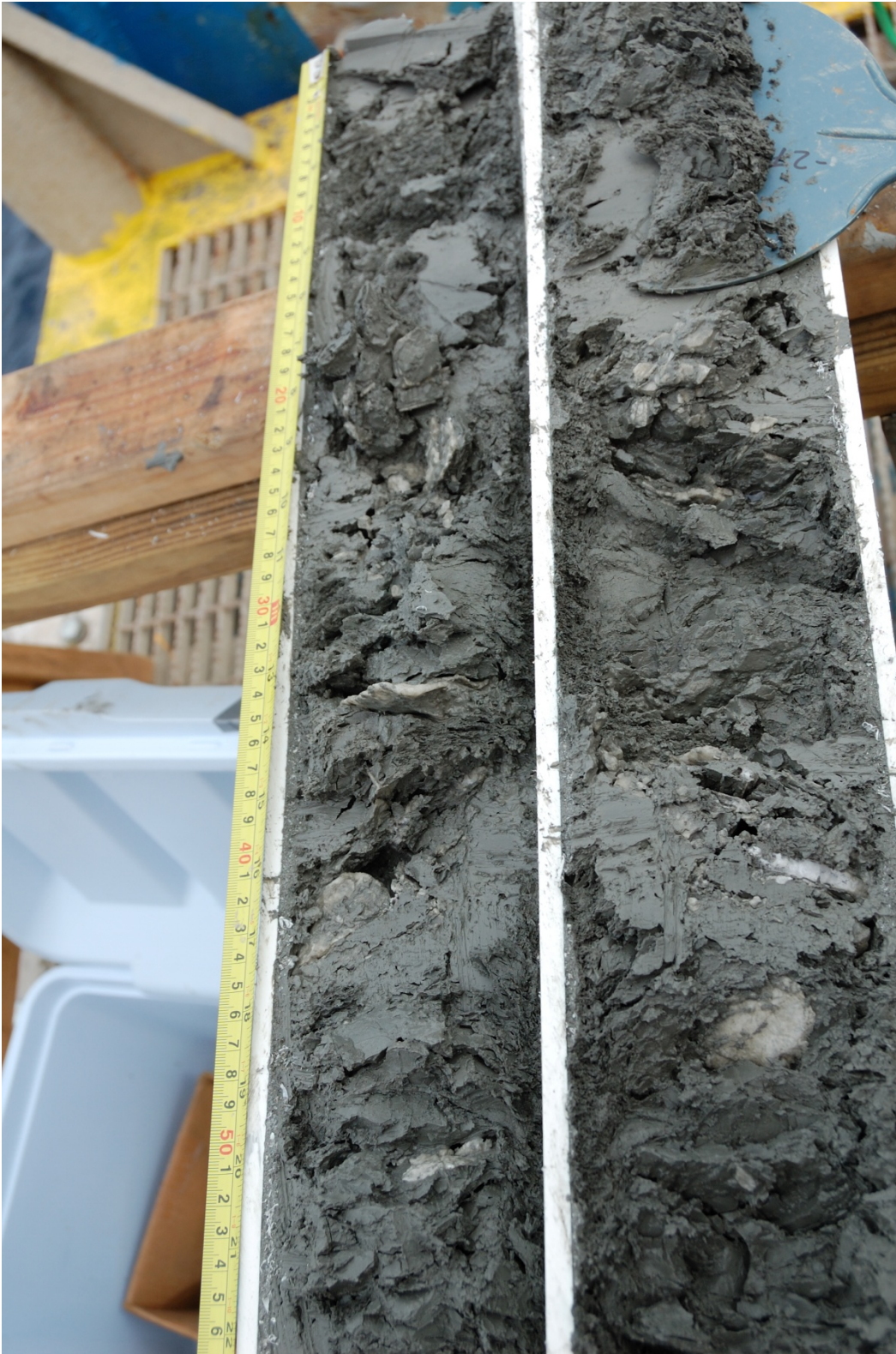
After 2 hours on deck, hydrate can still be observed in the bottom sections of JPC-001.
