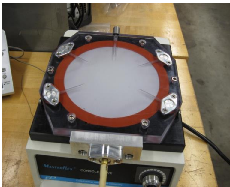
Figure 4. Filter assembly mounted on distilled water pumping station.
