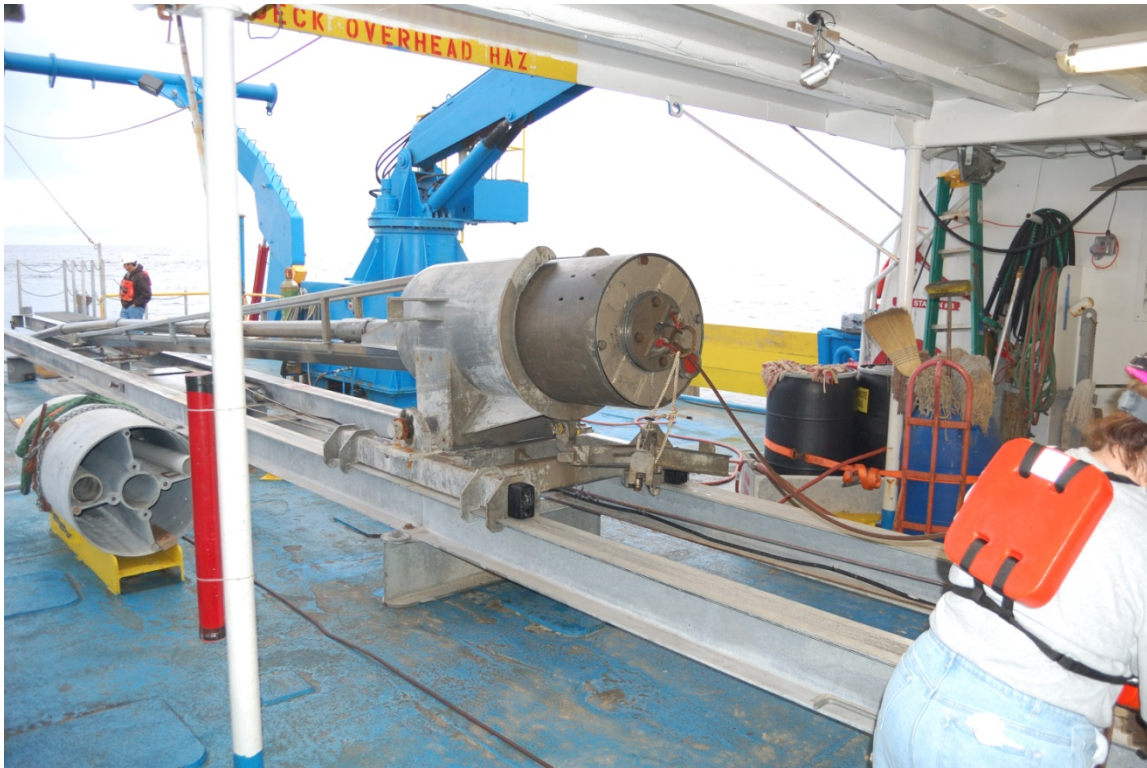
Recovery of the Jumbo Piston Corer to the deck.
