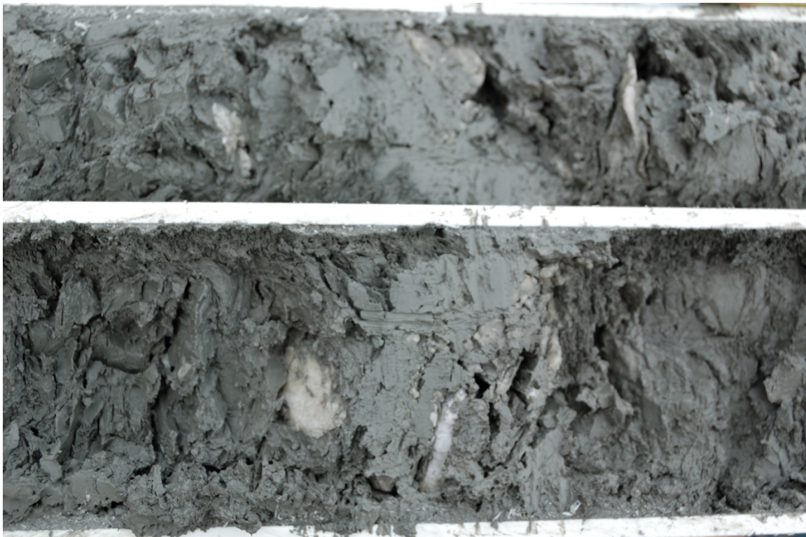
Extremely fine-grained material hosts hydrates at JPC-001 core-site.
