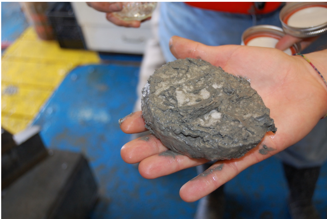
A disk of hydrates ~.8 in thick covered the entire cross-sectional area of JPC-001, 5.5 ft from the bottom of the core section.
