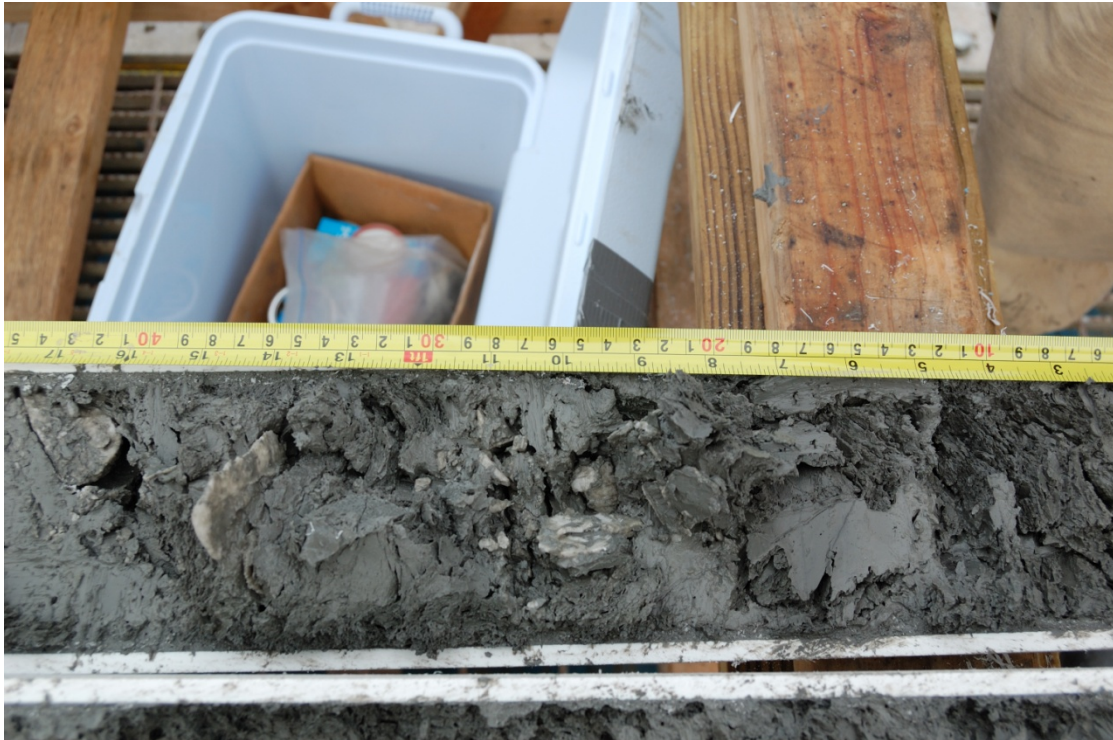
Bottom 3 ft section of JPC-001 contained hydrate nodules, blades, grains and granules.
