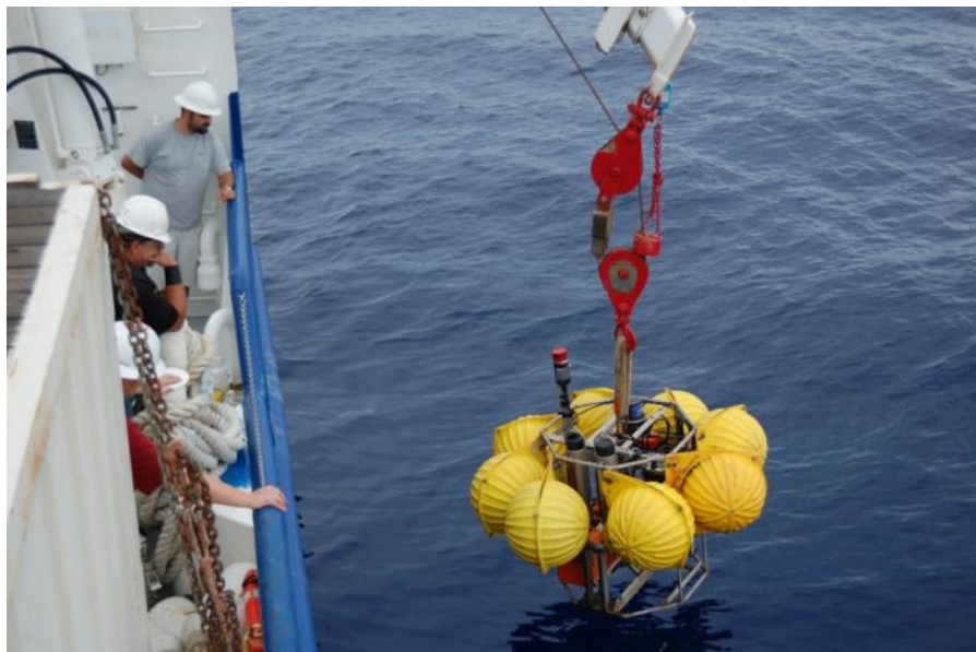
Figure 4. The ABIL is deployed using the Pelican's crane. Note the compact, central, arrangement of instruments - CTD, acoustic releases, battery, transponder - protected by the glass floats in hard-hats. Scanning sonar - red - is located above the other lander components for greater access to its surroundings.
