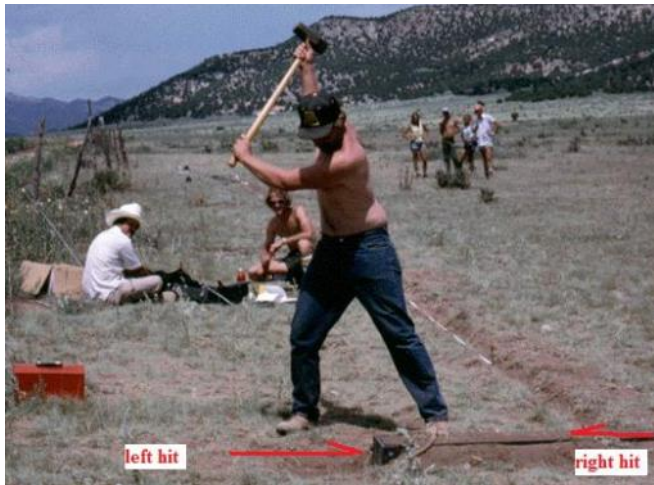
Figure 27. Using horizontal hits to generate S-waves.
