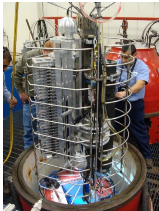
Figure 7. Loading the Lander into the SWRI pressure chamber.
